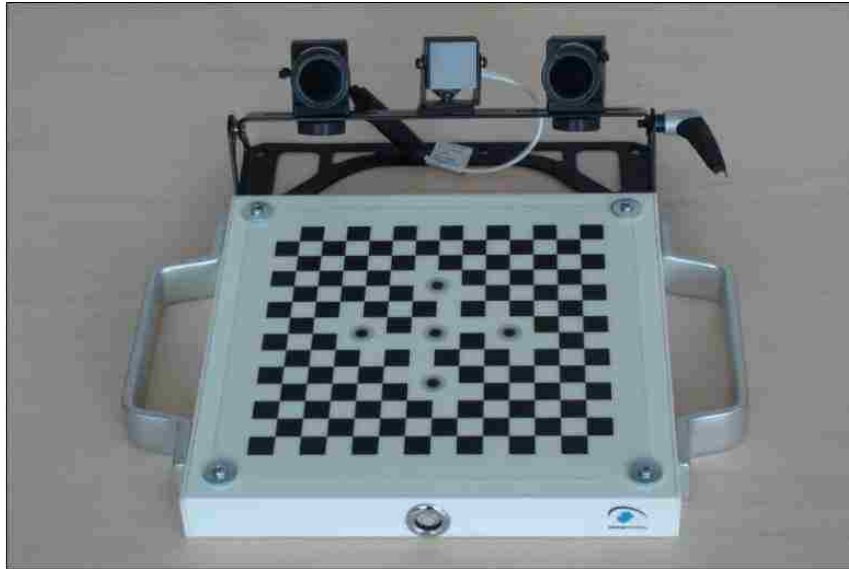
Figure 3.15 FaceLAB eye tracker cameras with calibration kit
